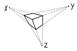
A cube has 3 sets of 4 parallel edges, and therefore a drawing of a cube needs 3 vanishing points. Choose an acute-angled triangle XYZ, and use the vertices as the vanishing points as shown. To then <u>see</u> the cube in perspective we must place the eye E in a position such that the lines EX, EY and EZ are parallel to the edges of the cube, which are perpendicular to each other. Therefore we define:
