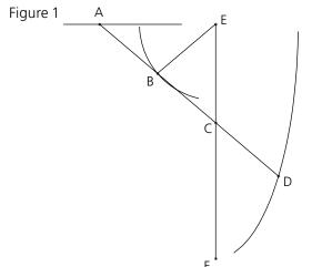
Here the door is represented by *AD*. The bar *EB* is free to rotate about the top of the door frame *E*, and a
