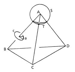
**Definition 4:** Given an edge AB, define the dihedral-angle of AB to be a/c, where c is the length of the circumference of a small disc centred on and perpendicular to AB, and a is the length of the arc cut off by the tetrahedron. Notice that 1 unit of dihedral angle equals 360 degrees.
