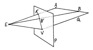
It suffices to prove that the image of one line, when extended, goes through V, because by the same proof they all will. Let AB be the line. Then EV is parallel to AB by definition 2, and therefore they both lie in a plane Q. The 3 points A', B' and V all lie in both the planes P and Q and hence on their line of intersection. Therefore extending A'B' along this line goes through V.
