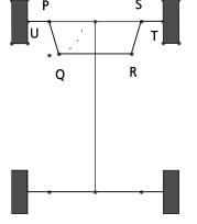
Now it is highly desirable that when taking a bend, the four circles to which the tyres are tangents should all have the same centre - otherwise the front tyres will soon lose their tread. The design problem is to choose *p* and *q* so that the point *V* of intersection of the stub axles produced lies as close to the line *AW* as possible for all positions of *Q*. Of course there also physical constraints on the maximum sizes of *p* and *q*.
