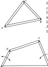
Make a triangle linkage from plastic geostrips or card strips using paper fasteners to join their ends. If you place the linkages on a table and fix AB then the point C or the triangle linkage is also
