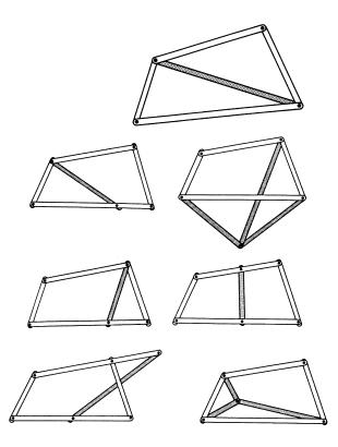
Having decided which of the above frameworks are rigid the investigation can be followed up by considering pentagonal or hexagonal frameworks. How about the following? Are any of them rigid? What is the minimum number of struts required to ensure that an ngon framework is rigid?
