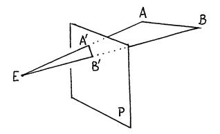
**Definition 1:** The image A' of a point A is where the ray EA pierces P. If also the image of B is B' then the image of the line AB is A'B'.
