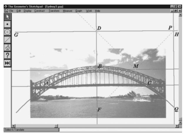
An alternative geometric model for the curved arch could just be a circular arc through *A*, *B* and *C* - how would you find its centre? Can you detect any visible difference between the parabolic and circular models? Some mathematical analysis, as well as further images, can be found at http://www.brantacan.co.uk/ and many other images at: http://architecture.about.com/ arts/architecture/
